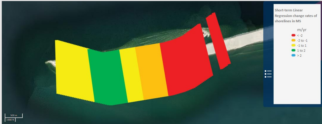
Figure 11: Short-term Linear Regression change rates of shoreline erosion for Ship Island, MS (Himmelstoss et al., 2017c).
