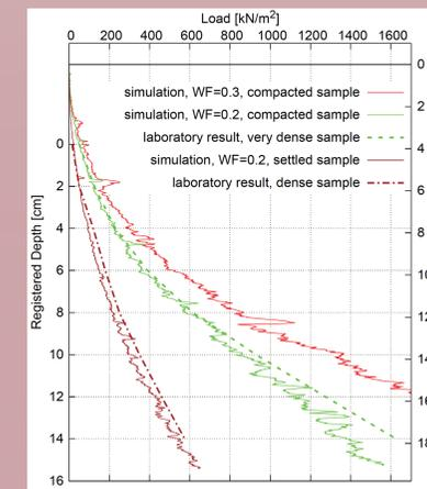
The soil sample was represented by 9.5 million spherical particles placed in a cylindrical mold. Rigid probe with cone-shaped tip was inserted with velocity 3cm/s. Simulations of probe insertion took ~10 days on 1152 cores. Parallel executions were performed on an SGI ICE X system having 3,456 nodes with 116 GB of DDR4-2133 RAM and two eighteen-core Intel Xeon E5-2699v3 processors, connected by 4x FDR InfiniBand network with Hypercube topology.
