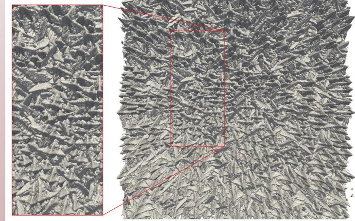
Growth of columnar dendrites in 1mm<sup>3</sup> domain was discretized with 3300 x 3300 x 3300 grid cells, or 36 billion grid points total and 4000 initial seeds [2]. Simulation was performed on 6400 cores Stampede, UTACC.
