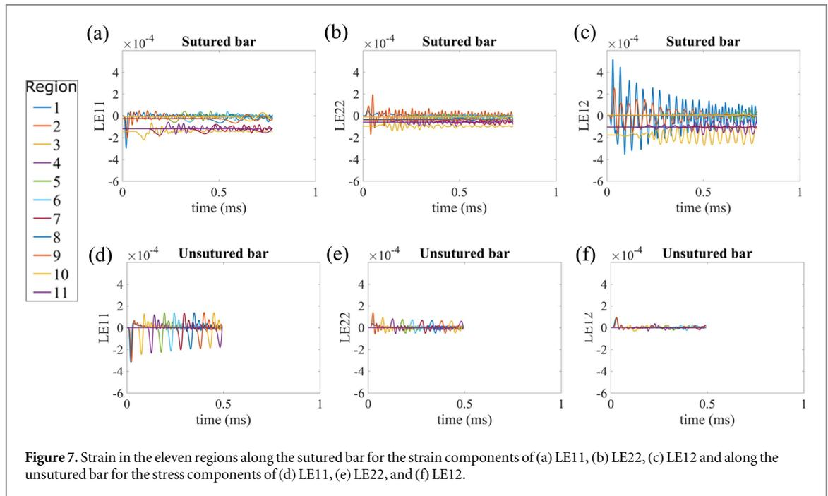
Figure 7. Strain in the eleven regions along the sutured bar for the strain components of (a) LE11, (b) LE22, (c) LE12 and along the unsutured bar for the stress components of (d) LE11, (e) LE22, and (f) LE12.
