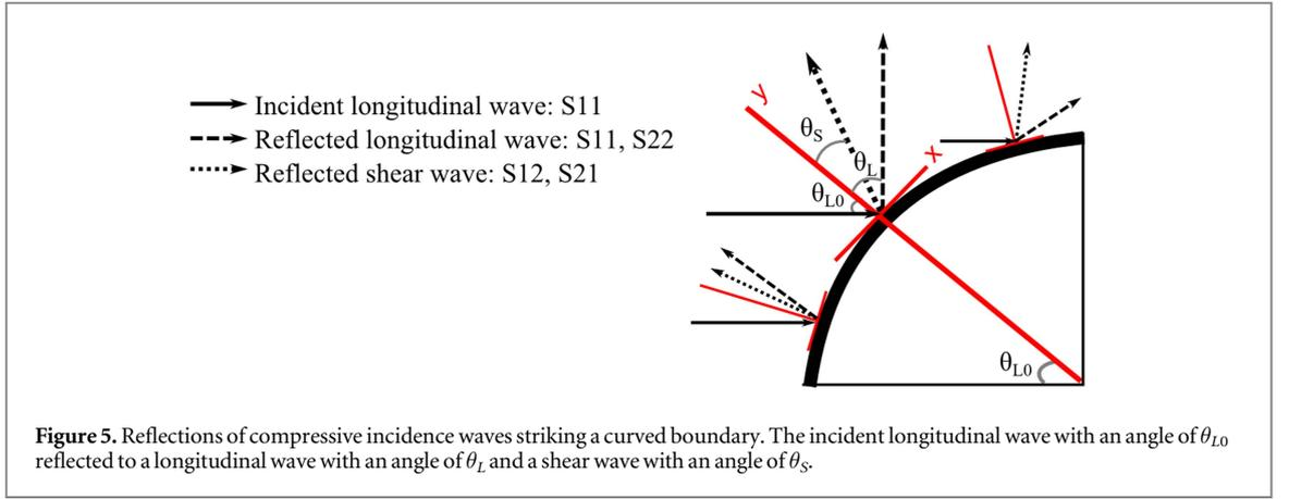
**Figure 5.** Reflections of compressive incidence waves striking a curved boundary. The incident longitudinal wave with an angle of  $\theta_{L0}$  reflected to a longitudinal wave with an angle of  $\theta_L$  and a shear wave with an angle of  $\theta_S$ .
