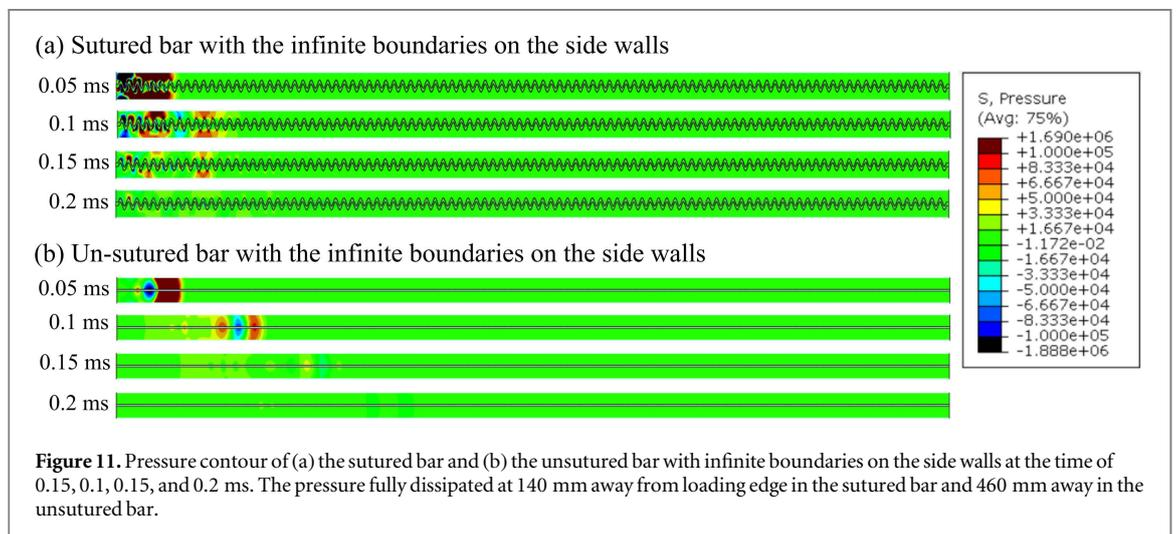
Figure 11. Pressure contour of (a) the sutured bar and (b) the unsutured bar with infinite boundaries on the side walls at the time of 0.15, 0.1, 0.15, and 0.2 ms. The pressure fully dissipated at 140 mm away from loading edge in the sutured bar and 460 mm away in the unsutured bar.
