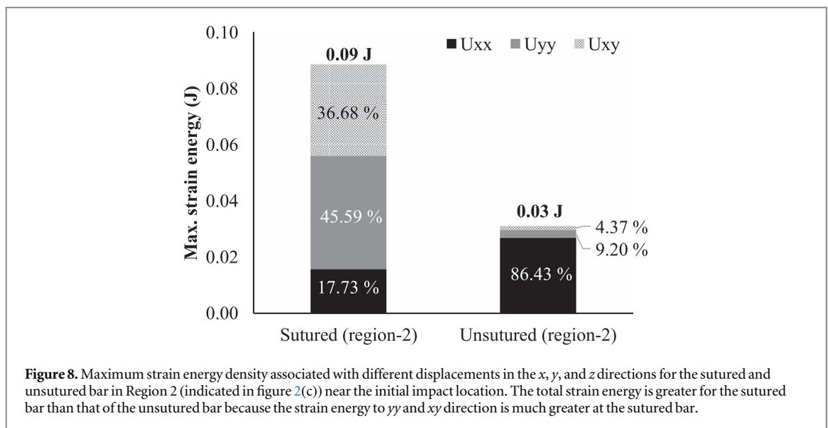
Figure 8. Maximum strain energy density associated with different displacements in the  $x$ ,  $y$ , and  $z$  directions for the sutured and unsutured bar in Region 2 (indicated in figure 2(c)) near the initial impact location. The total strain energy is greater for the sutured bar than that of the unsutured bar because the strain energy to  $yy$  and  $xy$  direction is much greater at the sutured bar.
