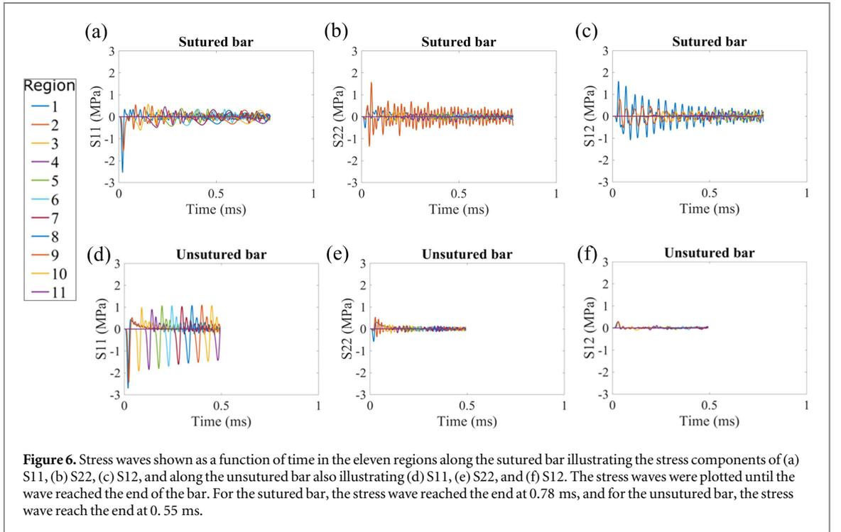
**Figure 6.** Stress waves shown as a function of time in the eleven regions along the sutured bar illustrating the stress components of (a) S11, (b) S22, (c) S12, and along the unsutured bar also illustrating (d) S11, (e) S22, and (f) S12. The stress waves were plotted until the wave reached the end of the bar. For the sutured bar, the stress wave reached the end at 0.78 ms, and for the unsutured bar, the stress wave reach the end at 0.55 ms.
