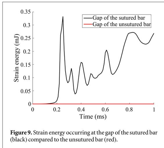
**Figure 9.** Strain energy occurring at the gap of the sutured bar (black) compared to the unsutured bar (red).
