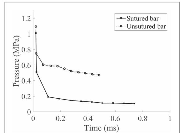
**Figure 4.** Comparison of pressure recorded along the sutured bar and unsutured bar. Each point represents the peak pressure at the eleven regions. The initial impact was 1 MPa, and the pressure when stress waves reached to the end was 0.47 MPa for the unsutured bar and 0.1 MPa for the sutured bar.
