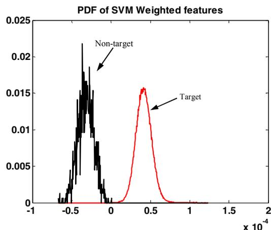
Figure 4. PDF of L-SVM statistic  $z$  for Experiment 4 (SNR = -10 dB).
