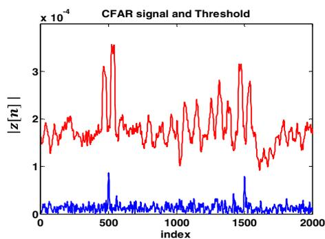
Figure 8. Example of signal and threshold values for experiment 5 for CFAR. The threshold is the upper curve. Targets are located at approximately indices  $n=500$  and  $1500$ .
