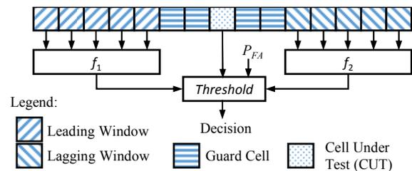
Figure 1. CFAR Processor Architecture.
