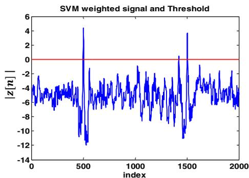
Figure 9. Example of signal and threshold values for experiment 5 for L-SVM method. The threshold is constant at zero. Note a false alarm just before index  $n=1500$ . Targets are located at approximately  $n=500$  and  $1500$ .
