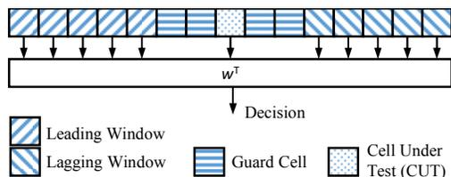
Figure 2. L-SVM Processor Architecture.
