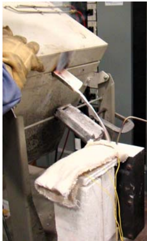
Figure 3. Pouring of casting type C.
