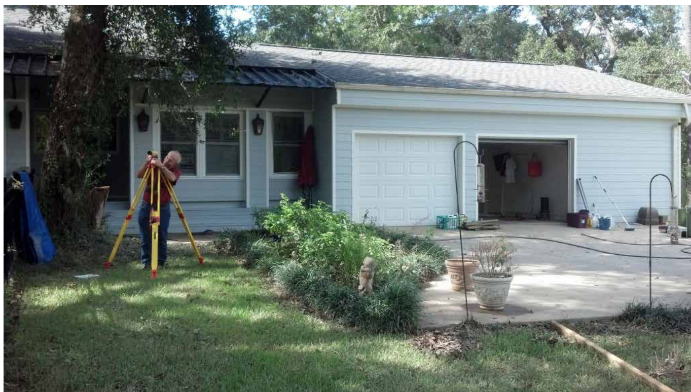
Figure 8. This home on Magnolia Dr. had a clear high water mark inside of the attached garage. Flood survey team members Marty Pope (pictured) and W. Scott Lincoln used this high water mark to help estimate the crest for the Wolf River at Bells Ferry Rd. (GLFM6) forecast point.
